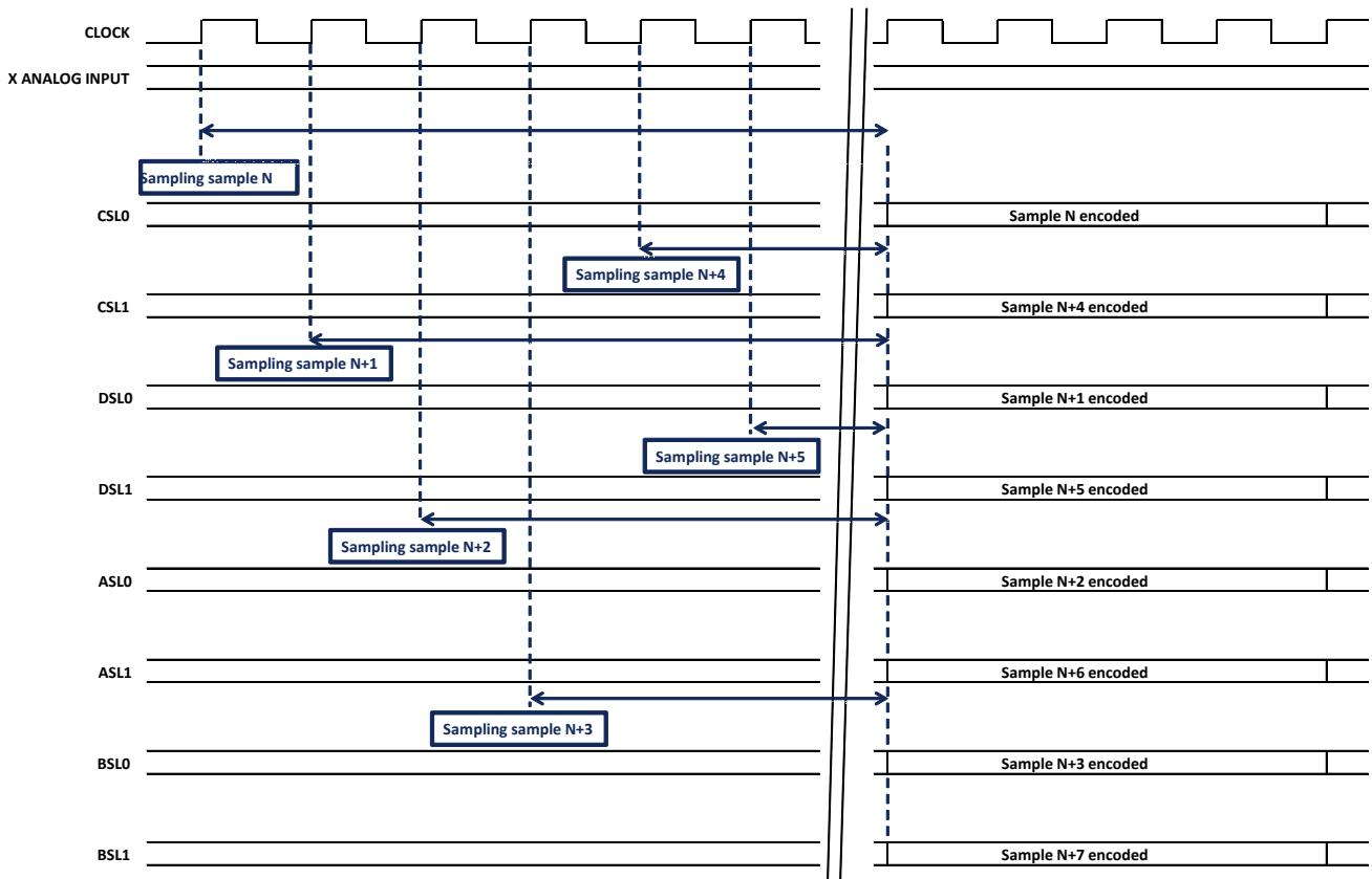
**Figure 19 - Timing diagram in serial interface in 1-channel mode**
