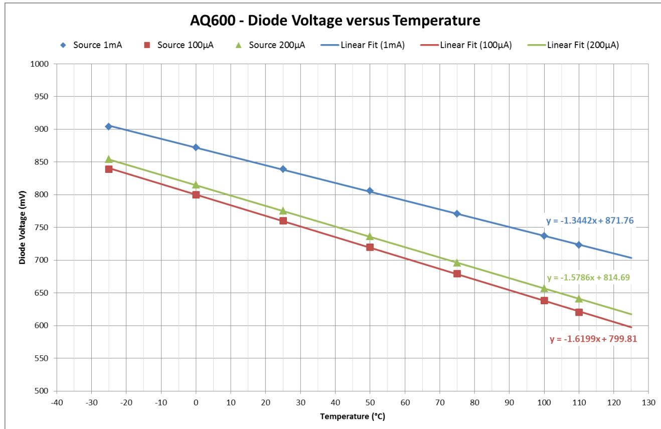
**Figure 26: Diode voltage vs temperature for 3 different input currents (blue: 1mA, green: 200µA, red: 100µA)**
