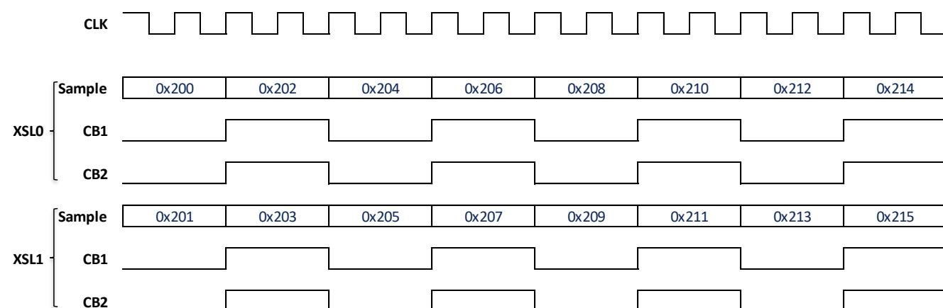
**Figure 24 – Chronogram of the Ramp test mode**
