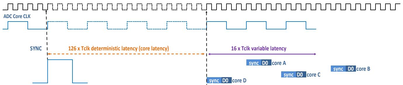
**Figure 3 - Deterministic (core conversion) latency and non-deterministic (serial output) latency**
