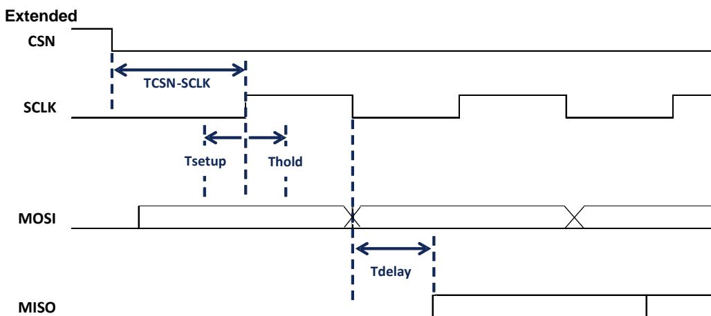
**Figure 5 - SPI timing diagram**
