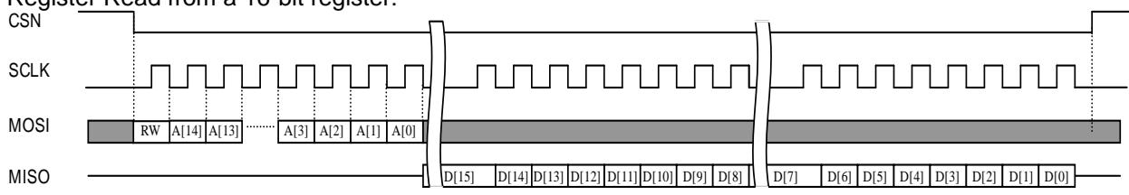
**Figure 12 - SPI reading**
