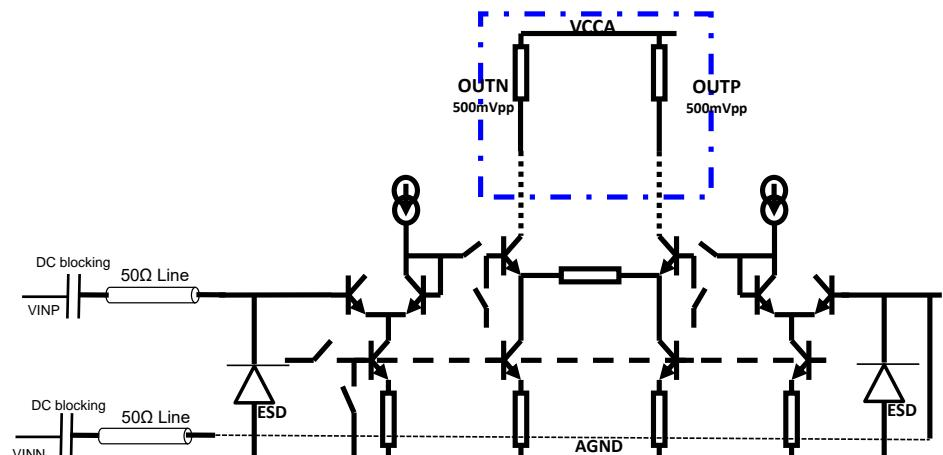
**Figure 2 – Analog input scheme regarding max ratings**
