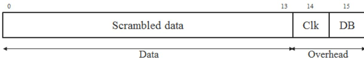
Figure 33 - Frame format after encoding
