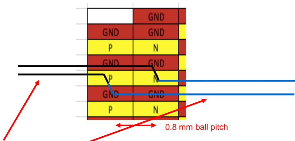
Length on board + length on package are almost the same on N and P (less routing on board for P results from more routing inside package for P).
