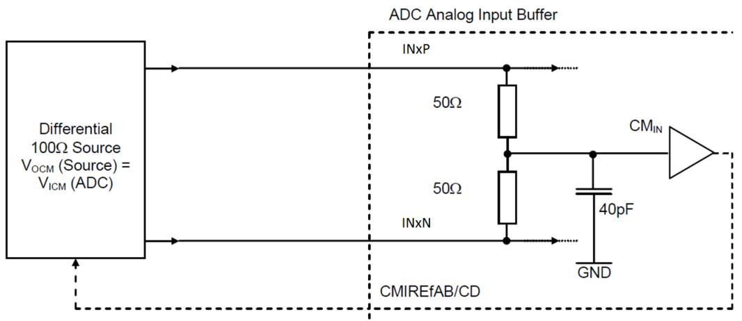
**Figure 28 : Differential analog input implementation (DC coupled)**
