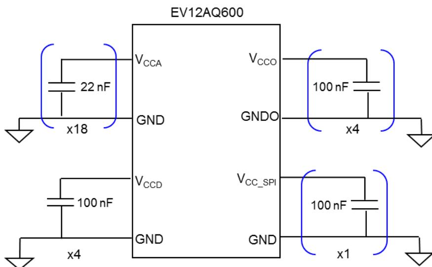
**Figure 30 - Power Supplies decoupling scheme**
