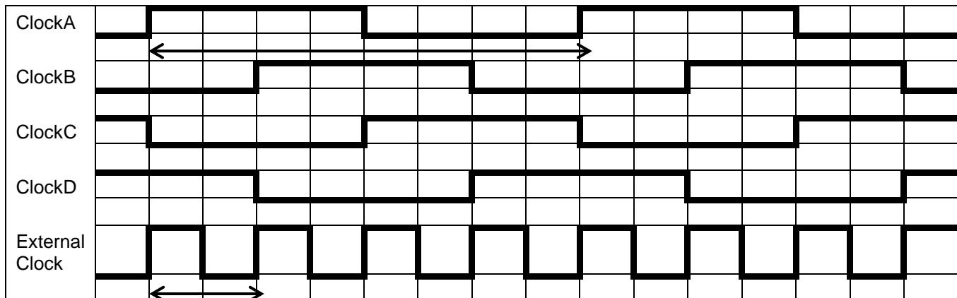
Figure 15 - Clocks for four cores interleaved
