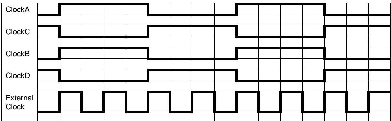
**Figure 17 - Clocks for two cores interleaving – configuration 1: Interleaved of A and B, and interleaved of C and D CLK\_MODE\_SEL = 1**
