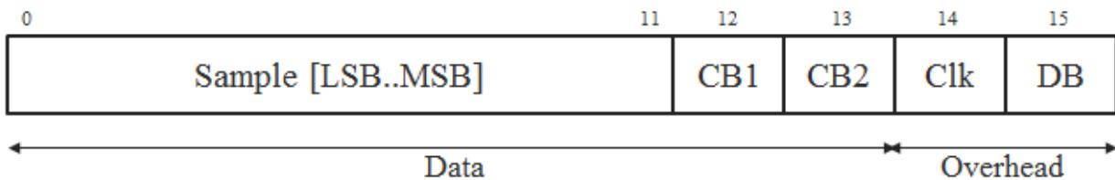
Figure 31 - ESIstream frame with EV12AQ600
