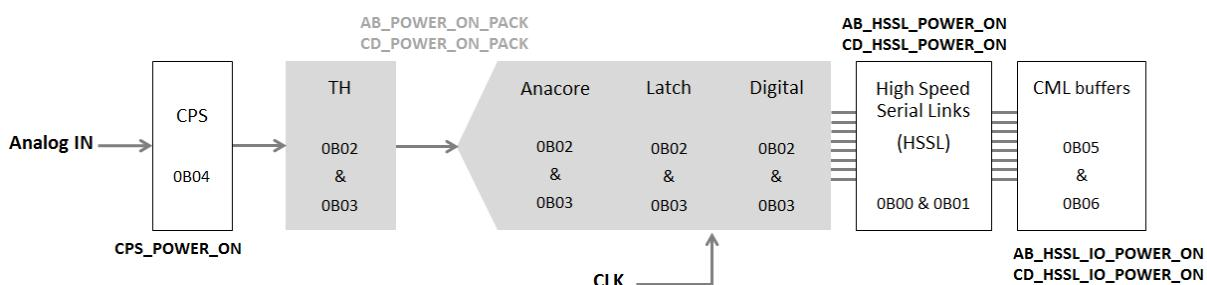
**Figure 29 : Internal blocks that can be powered ON or OFF and their respective register addresses.**
