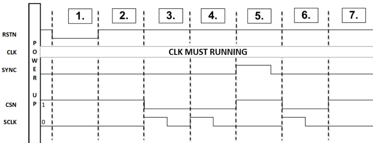
**Figure 13 – Start-up sequence when using the SPI interface**
