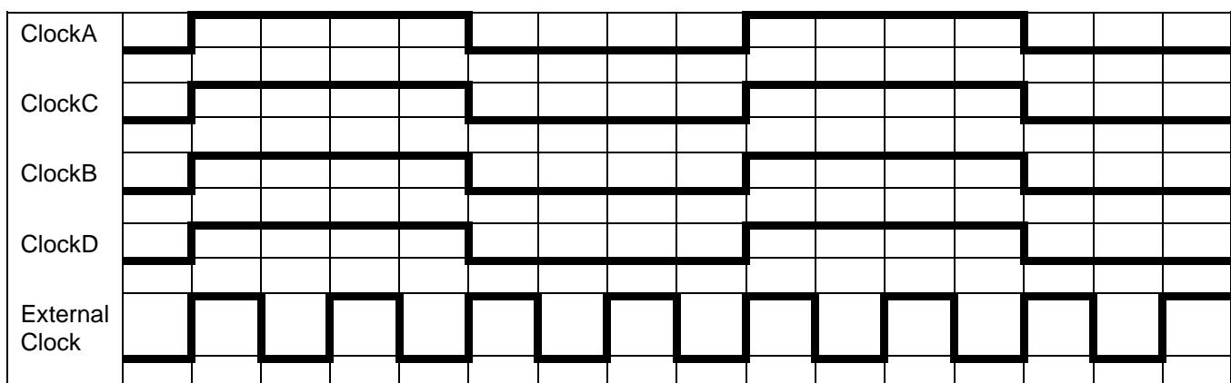
Figure 16 - Clocks for four cores aligned: averaging or four channels, CLK\_MODE\_SEL = 3
