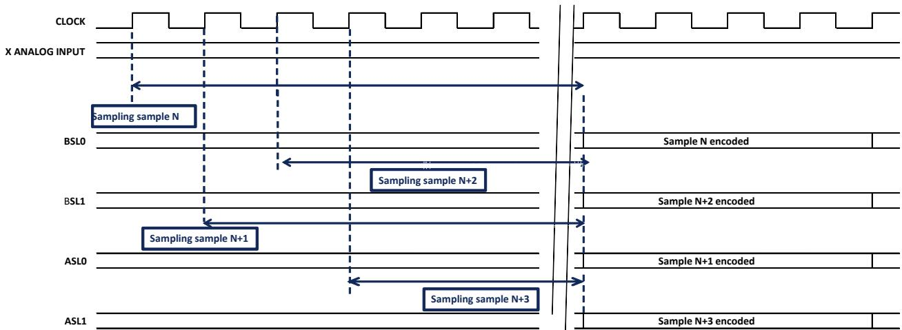
**Figure 20 - Timing diagram in serial interface in 2-channel mode**
