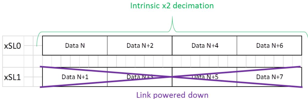
Figure 22: Powering down 1 link gives a x2 decimation.
