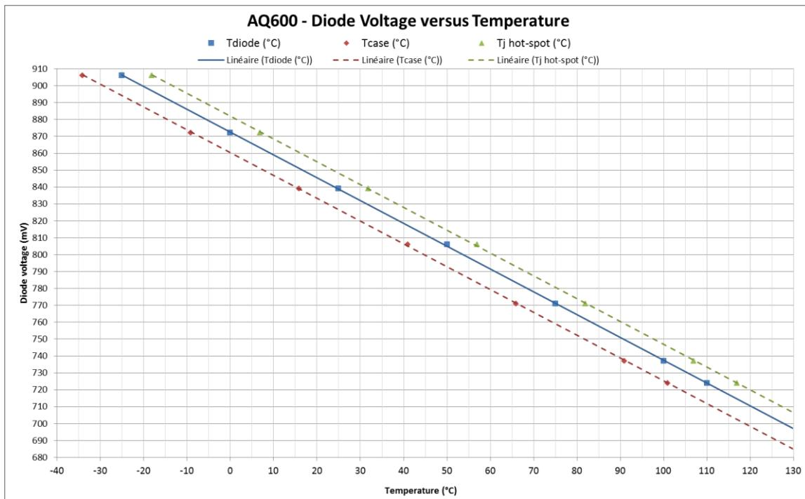
Figure 27: Voltage vs temperature. Blue=diode voltage - Green=hot-spot junction voltage- Red=case voltage.
