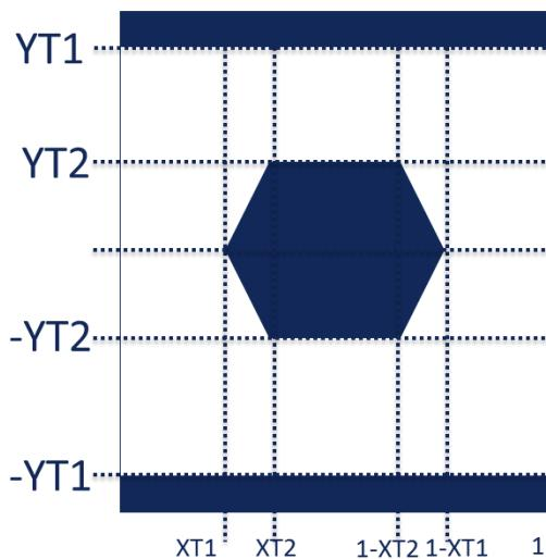
**Figure 4 - Serial link eye diagram**
