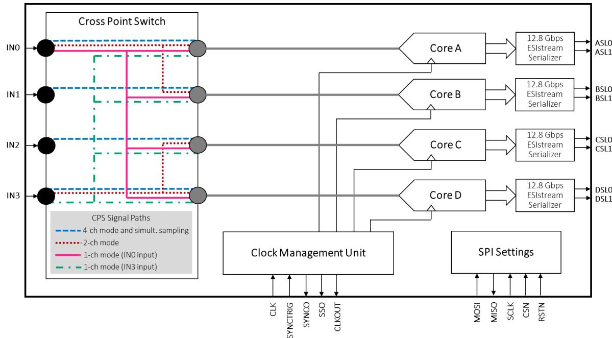
**Figure 1 - Quad 12-bit ADC with 12.8 Gbps serial link**
