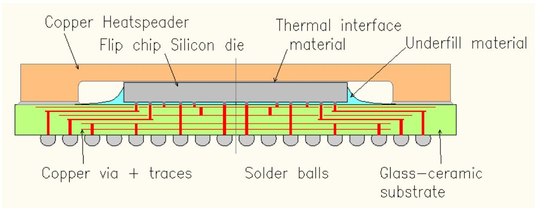
Figure 6 – Package cross-section
