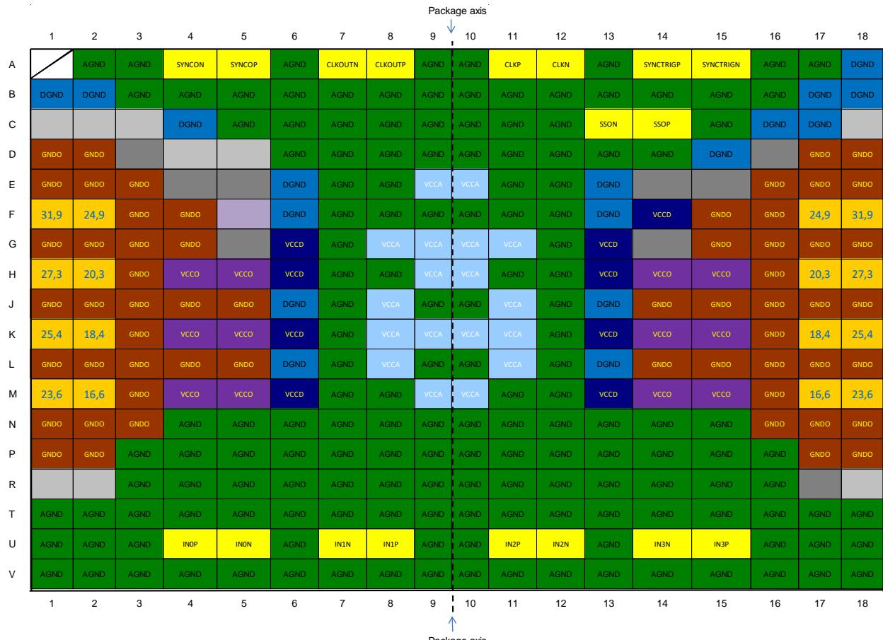
Figure 10 – Skew mapping (values are in ps)
