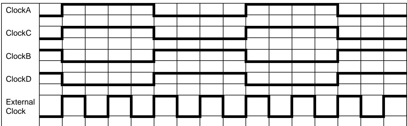
**Figure 18 - Clocks for two cores interleaving – configuration 2: Interleaving of A and C, and interleaving of B and D CLK\_MODE\_SEL = 2**
