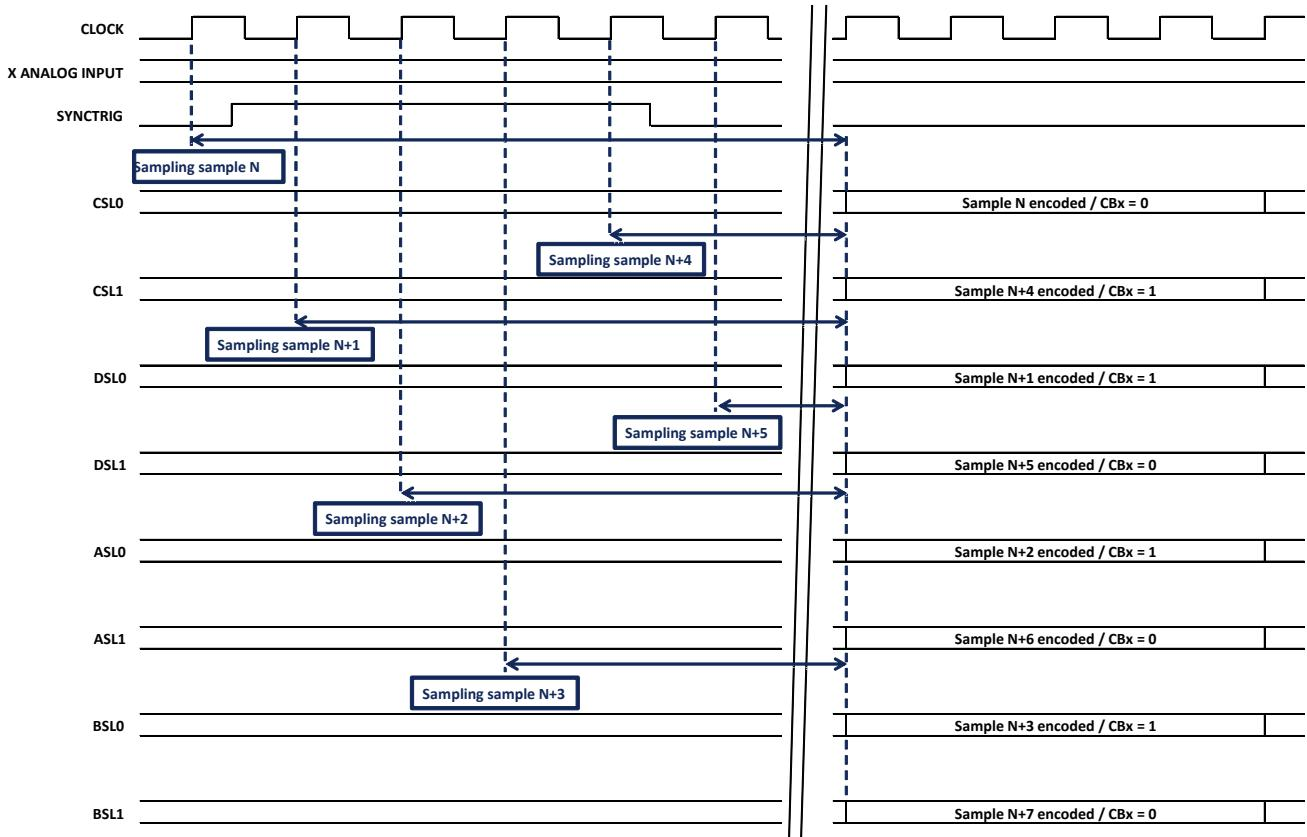
**Figure 23 - Trigger mode timing diagram in serial interface**
