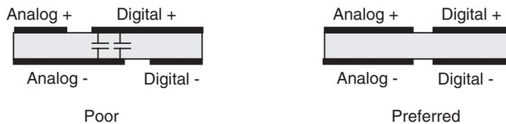
Power planes are designed using the same rules as ground planes. Keep the analog supply plane entirely under the analog ground plane, see on [Figure 2-5: Preferred](#). This gives an analog supply plane over the analog ground plane and a digital supply plane over the digital ground plane. In this case, it could not cause unwanted capacitance between the two planes.
