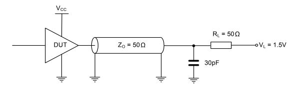
Figure 3. Test Loads specific to TWLQZ, TWHQX, TELQX, TEHQZ, TGLQX, TGHQZ
