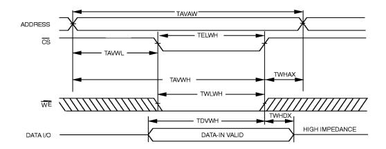
Note: The internal write time of the memory is defined by the overlap of  $\overline{\text{CS}}$  Low and  $\overline{\text{W}}$  LOW. Both signals must be activated to initiate a write and either signal can terminate a write by going in active mode. The data input setup and hold timing should be referenced to the active edge of the signal that terminates the write.
