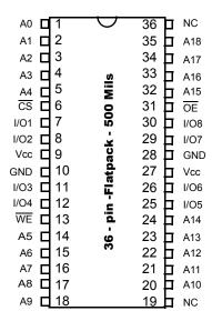
Note: NC pins are not bonded internally. So, they can be connected to GND or Vcc.
