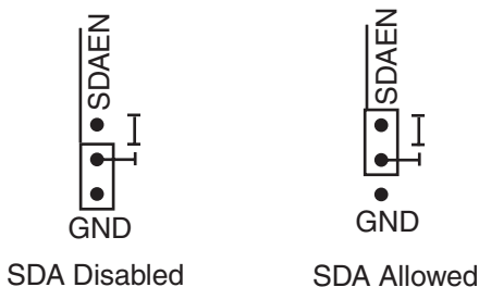
Figure 4-5. DC SDAEN Jumper Settings
