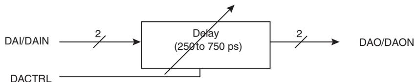
The input buffer for DAI/DAIN is described in Figure 4-4. As it is on-chip already +2 x 50Ω terminated the 100Ω LVDS external termination is not required.
